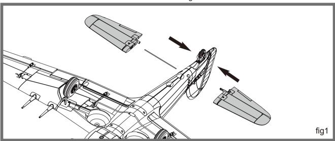
2. Secure the horizontal tail piece in place using the include screw: PA2.6\*10. Use caution to avoid over-tightening the screw.
